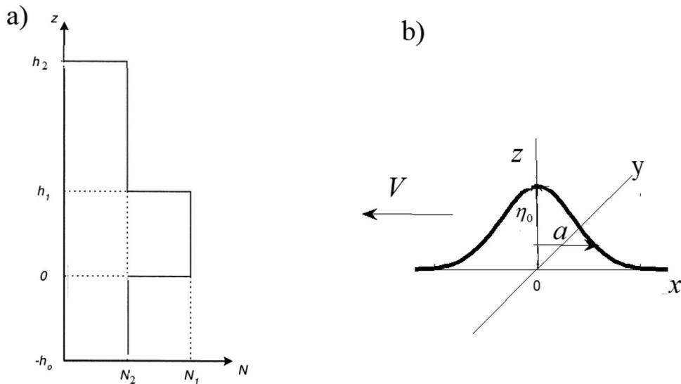
Fig. 2. (a) A model of the vertical profile of the BV-frequency  $N(z)$  in the ocean. The layer  $0 < z < h_1$  represents the thermocline, which has a maximum BV-frequency  $N_1 \gg N_2$ . (b) An idealized perturbation to the thermocline (at  $z=0$ ), having a vertical displacement  $z = \eta(x + Vt, y)$  and characteristic horizontal scale  $a$ . The perturbation is shown moving to the left at velocity  $V$ .
