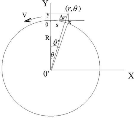
Fig. 5. Diagram of transition from rectangular coordinate system  $(x, y)$  to the local curvilinear coordinate system  $(r, \theta)$  near the perimeter of the circle.
