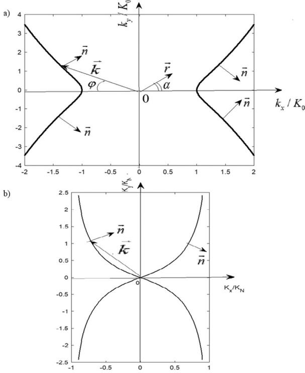
*Fig. 3.* Wave number curves relating wave number components  $k_x$  and  $k_y$  of the wave number vector  $\vec{k}$  of stationary internal waves generated by a horizontally moving (to the left) source with speed  $V$ . (a) Case of the thin stably stratified layer with  $N = N_1$  inside the deep water ( $\mu_1 h_1 \ll 1$ ,  $kh_0 \gg 1$ ,  $k\Delta h \gg 1$ ). (b) Case of the stably stratified layer in the shallow water ( $k\Delta h \ll 1$  and  $\mu_2 h_0 \ll 1$ ).
